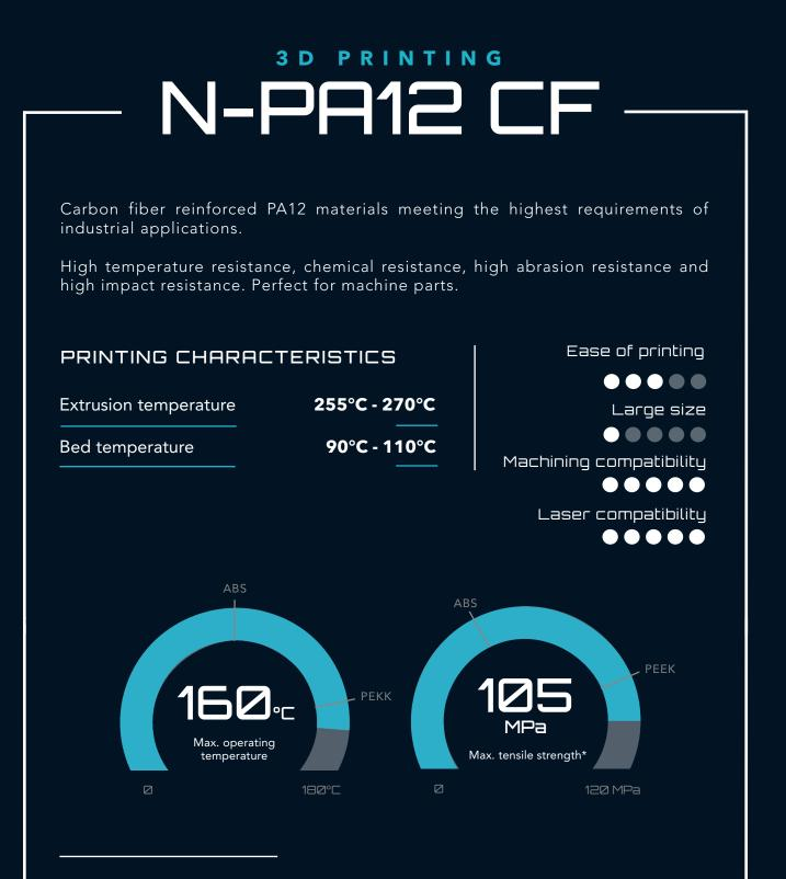
We recommend storing your spools in a dry, dark place, if possible with desiccant. To ensure perfect printing, we recommend steaming your filament at 60°C for 4 hours or more, when the spool has been exposed to the open air for a long period.
